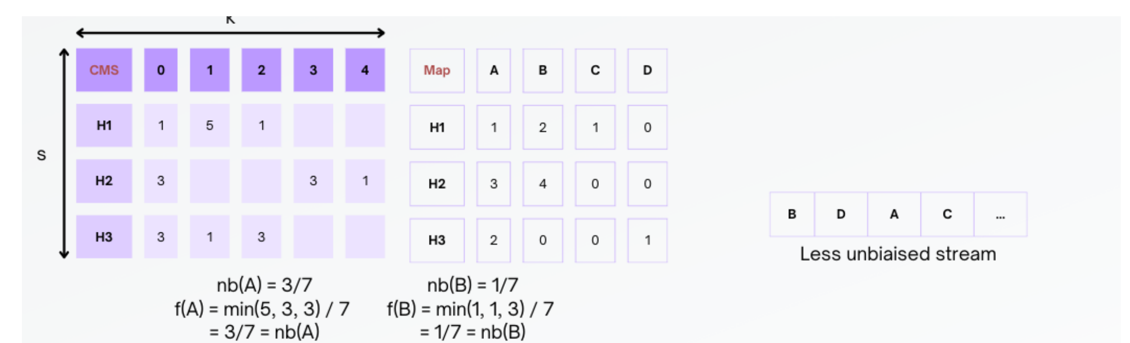
Figure 5: Use of Count Min sketch to unbiased a stream
